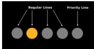
Fig. 1: Virtual (iPad) button display for answering incoming ATC messages. (The second button is yellow to indicate it is active)
